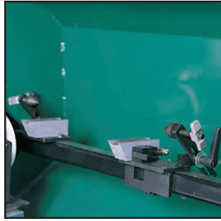
Bedbar Mounting System combines magnetic set-up planes with easy-adjust center supports. This provides a solid surface and holding of the bedbar during the set-up and grinding processes.
