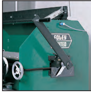
Fast Set-Up in determining front face and top face angles for the bedknife. Match the manufacturer's specifications by rotating the lever between the front and top face angles.
