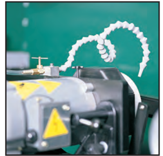
Flood Coolant System is integral to the machine. A self-contained water pump system filters and re-circulates the water. Water flow is controlled by the operator and the flexible water tubing allows for easy positioning.
