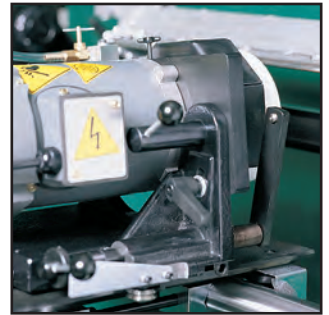
Diamond Wheel Dresser allows the operator to redress the grinding wheel. The permanently attached dresser stores easily out of the way during grinding and requires minimal adjustments for dressing.
